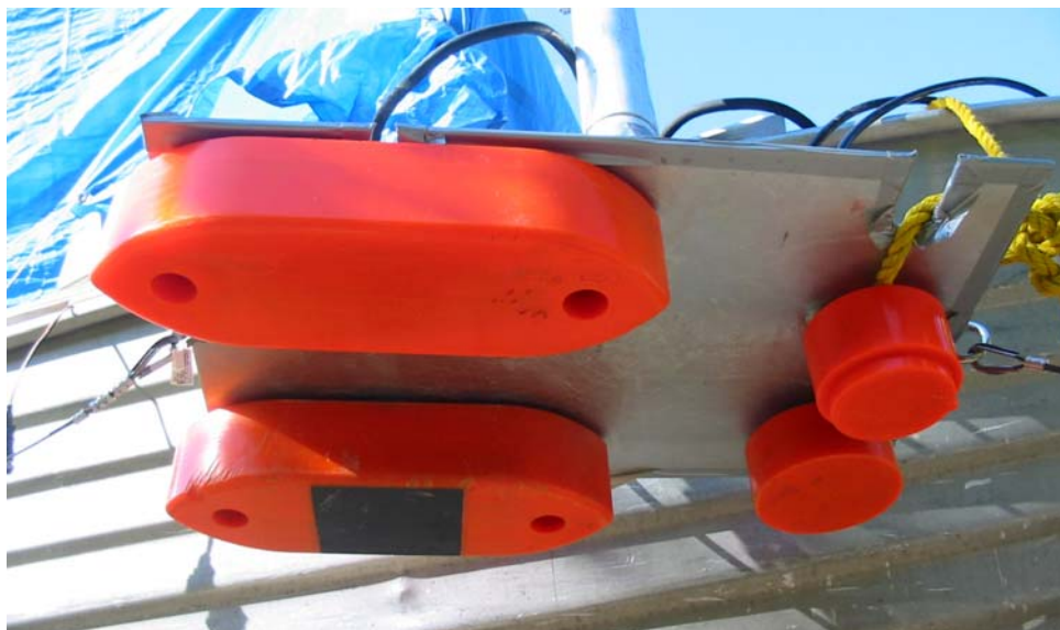
Figure 3: Image of the Simrad split-beam transducers mounted on an aluminum plate. The transducer array was deployed ~50 cm below the surface on the forward starboard gunwale of the survey vessel. Transducers shown are; forward left – 120 kHz (4.4° X 9.0°), rear left - 70 kHz 11° X 11°, forward right - 200 kHz 7° X 7°, and rear right - 120 kHz 7° X 7°. Not shown is the 710 kHz 5°X5° transducer.
