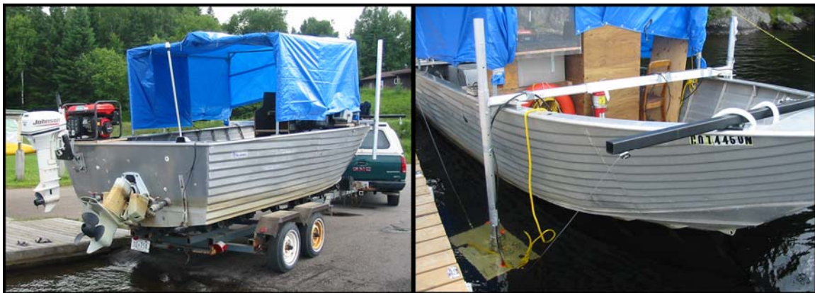
Figure 1a & b: Acoustic survey vessel “Henley” outfitted with split- beam and multi-beam hydroacoustic systems. The transducers were deployed off of aluminum poles on the forward port and starboard gunwales. A reinforced cross-beam with aluminum tubes were welded on each end to allow the depth of the transducers to be adjusted.
